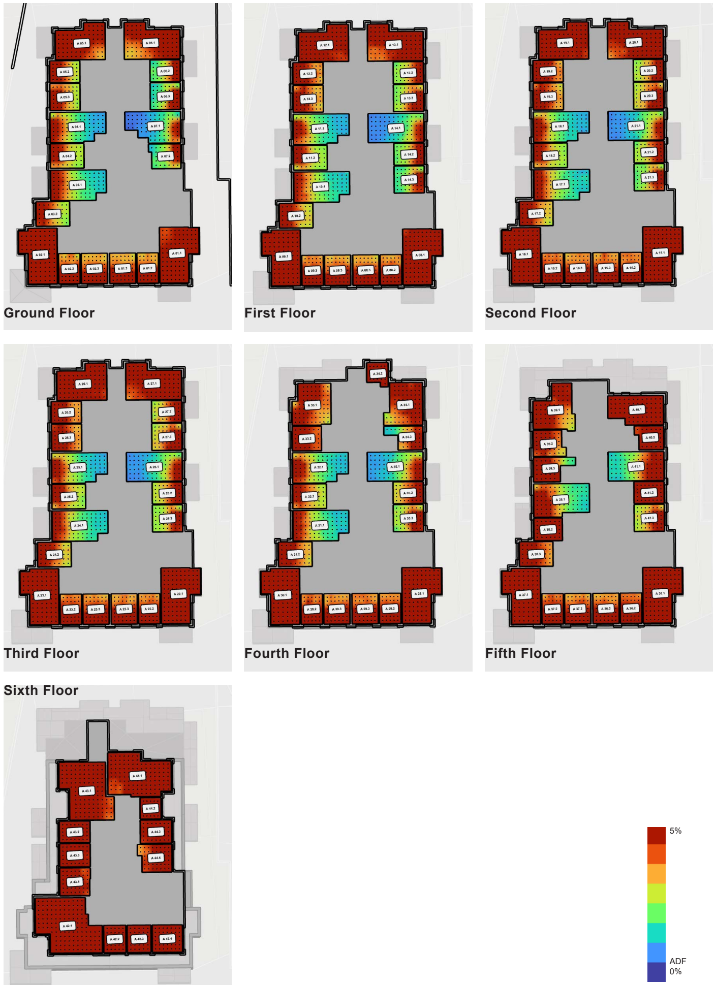
Figure 33: Block A - Ground to sixth floor false colour plans of ADF. Scale 0 - 5%
