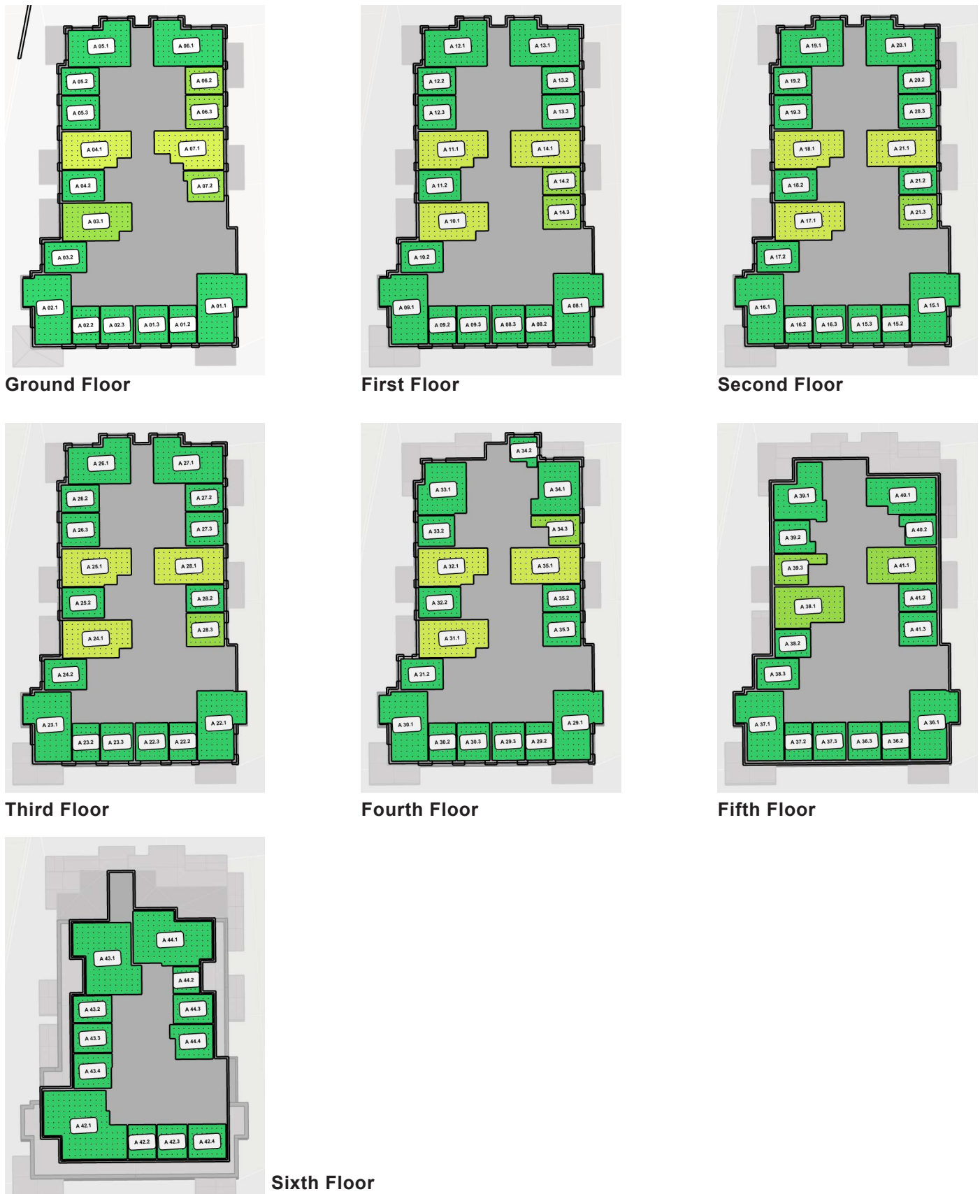
Figure 36: Block A - Daylight Provision to habitable rooms on all floors.
