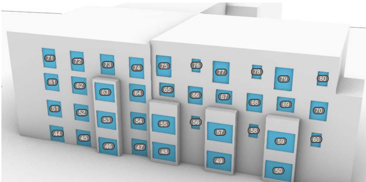
Figure 10: Carracail Apartments - View of model's North Elevation of showing location of windows assessed for VSC.
