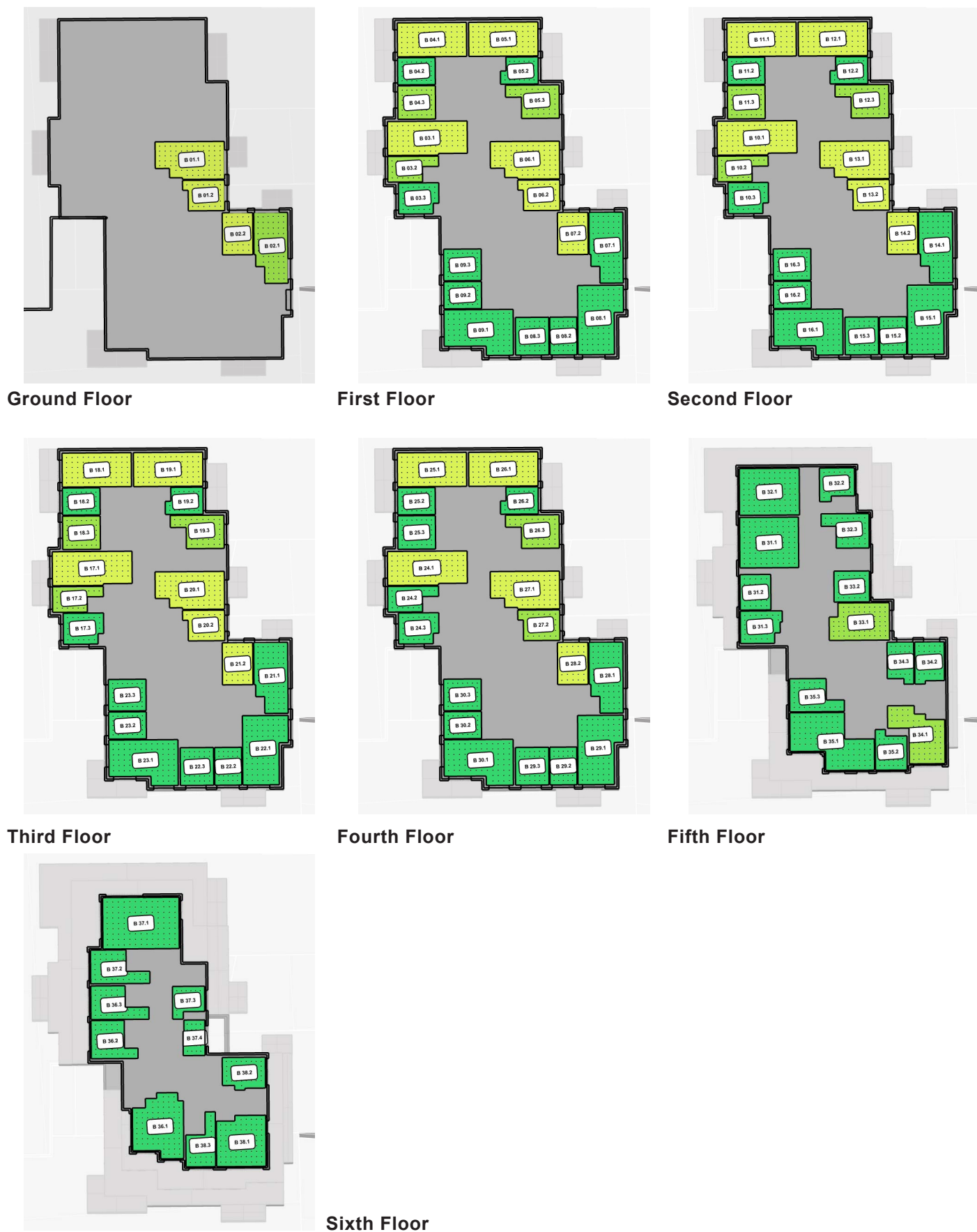
Figure 37: Block B - Daylight Provision to habitable rooms on all floors.
