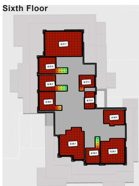
Figure 34: Block B - Ground to sixth floor false colour plans of ADF. Scale 0 - 5%
