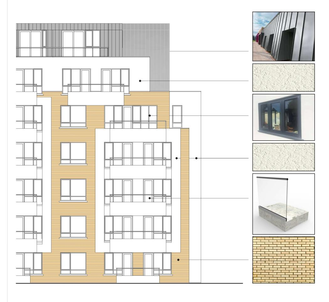
TYPICAL ELEVATION PROPOSED FINISHES
