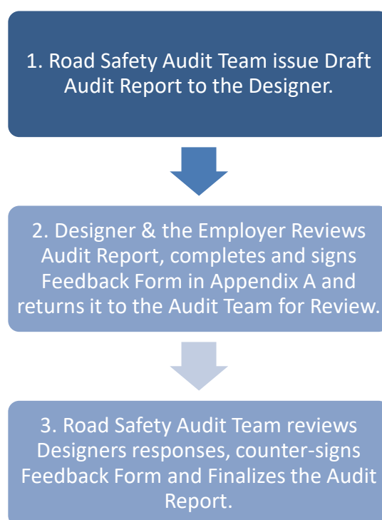
Figure 5.1 – Road Safety Audit Sign-Off and Completion Process
